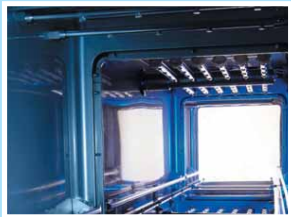
Washing chamber without internal pipes.
