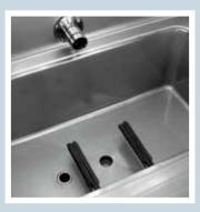
A one piece deep drawn pressed tank with fully rounded corners, sloped towards the drain to prevent dirt build up, provides fast drainage in only a few minutes. Pressed tanks, with no welded points offer a guaranteed water tight solution.
