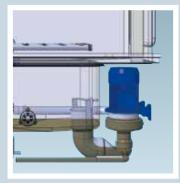
Self-draining wash pumps provide maximum hygiene with no smells and all wash and rinse zones drain automatically at the push of a button.
